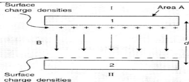
Electric field between the plates of capacitor
